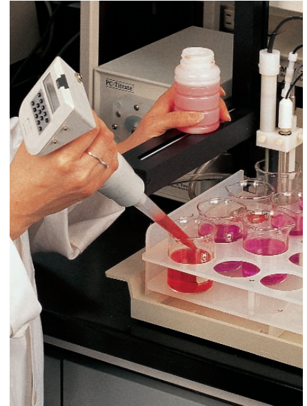
Several in-depth tests are performed on coolant samples to determine the health of the cooling system.
