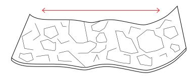
2. On a clean bench, cut vertically down to open up the filter.
