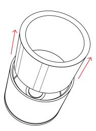
1. Remove used COF filter paper from unit per Caterpillar Operation and Maintenance Manual instructions.
