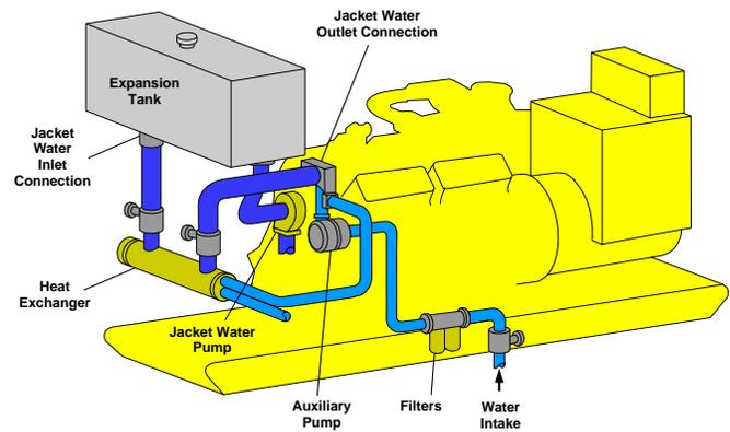
**Fig. 3: Schematic of typical heat exchanger cooling system.**
