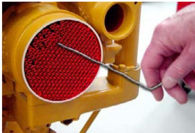
Fig. 74: Cleaning the tube bundles.
