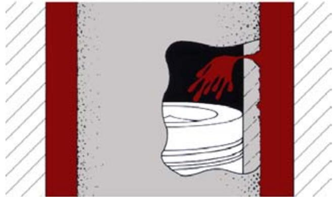
Fig. 47: Eventually, a pit can penetrate the cylinder wall and allow coolant to leak into the cylinder.
