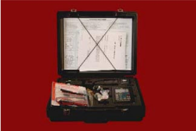
**Fig. 100: Multitach to Check Fan and Engine Speed.**
