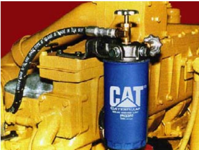
**Fig. 36: Supplemental Coolant Additive Element Assembly.**
