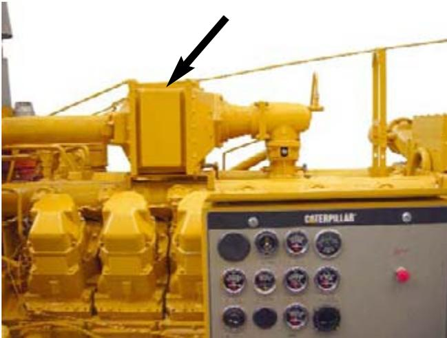
Fig. 8: One type of aftercooler.
