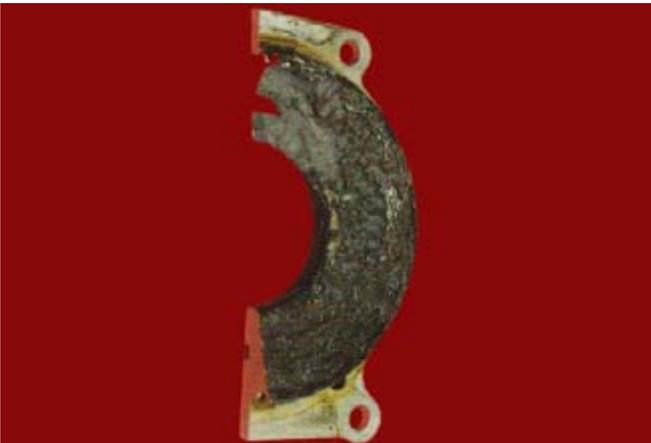
Fig. 49: Corrosion/erosion of aluminum Water Pump Adapter .
