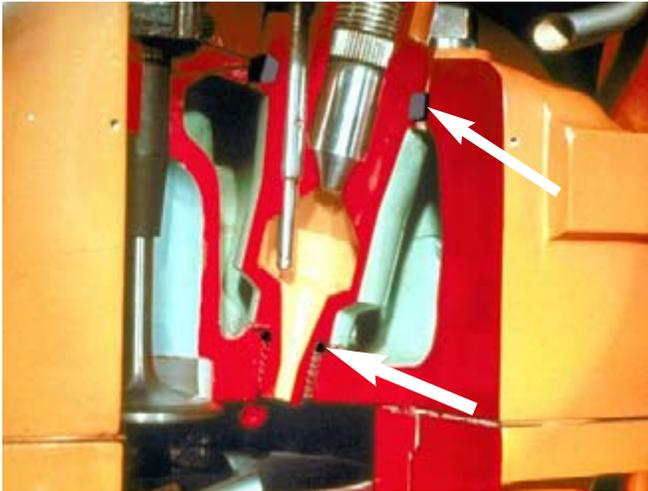
**Fig. 79: O-ring seals and gasket on precombustion chamber.**
