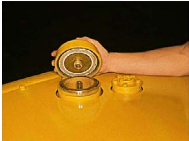
Fig. 63: Type of radiator cap held by studs.
