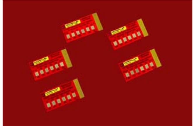
Fig. 98: Adhesive cards for Varied Temperature Ranges.
