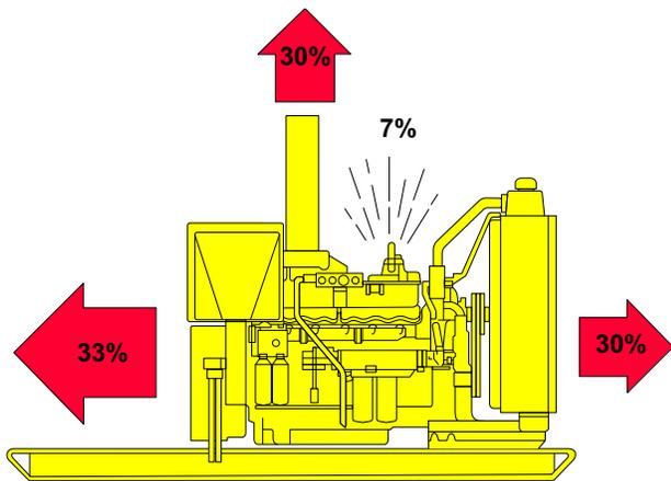
Fig. 1: Proportional amount of heat dissipated from engine.
