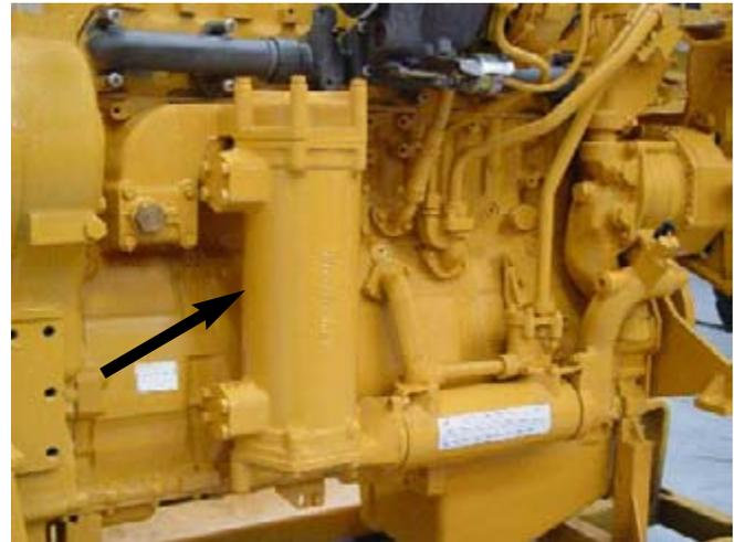
Fig. 9: Typical transmission oil cooler.
