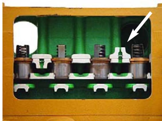
Fig. 68: Bleed hole in water temperature regulator housing.
