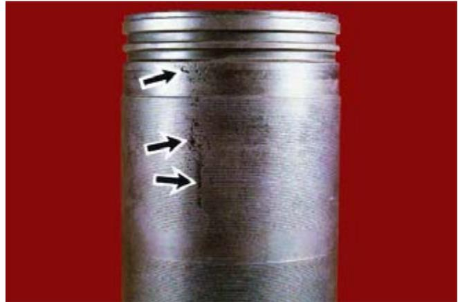
Fig. 44: Example of cylinder wall cavitation-erosion.
