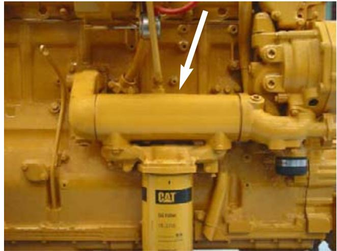
Fig. 7: Typical engine oil cooler.
