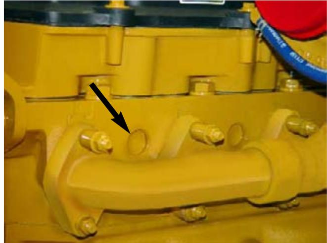
**Fig. 78:** Freeze plug in cylinder head.
