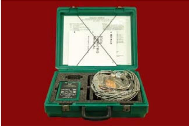
Fig.96: Five Channel Digital Thermometer Group.
