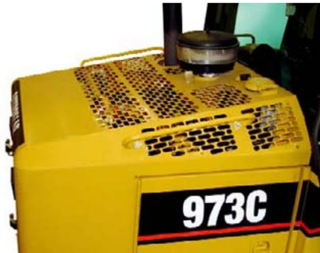
Fig. 108: Perforated Hood and Engine Side Enclosures.
