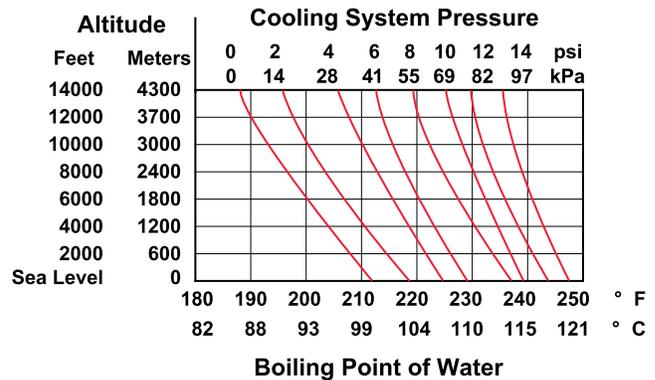
Fig 5: Pressure/temperature chart.
