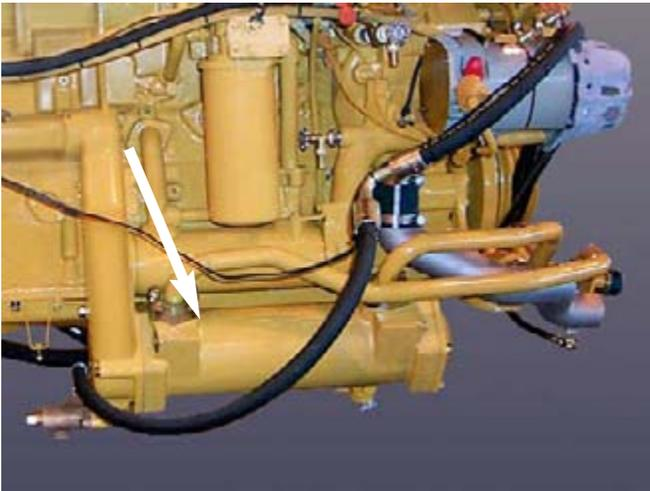
Fig. 10: Combination retarder/transmission oil cooler.
