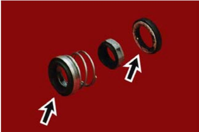
Fig. 38: Water Pump Seal Deterioration.
